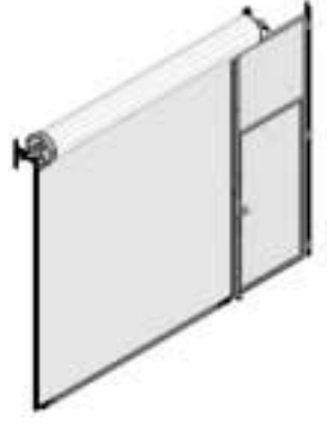
> Wicket Door For personal access, and added efficiency and convenience
